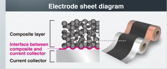
Isolating and calculating composite layer resistivity and interface resistance using inverse problem analysis
