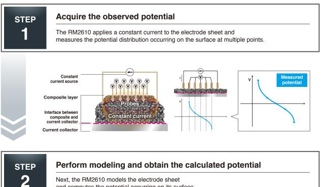
Next, the RM2610 models the electrode sheet and computes the potential occurring on its surface.
