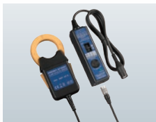
CLAMP ON AC/DC SENSOR CT9691-90 φ35mm, AC/DC 100 A, Accuracy: ±1.5%rdg.±1.0%f.s. (DC, 45 to 66Hz) Cord length 2 m (6.56 ft)
