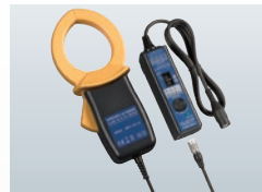
CLAMP ON AC/DC SENSOR CT9693-90 φ55mm, AC/DC 2000 A, Accuracy: ±2.0%rdg.±0.5%f.s. (DC) ±1.5%rdg.±0.5%f.s. (45 to 66Hz) Cord length 2 m (6.56 ft)
