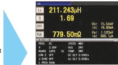
L, Q and Rdc continuous measurement screen L and Q (1 kHz, 1 mA constant current measurement) and Rdc (DC measurement) display screen
