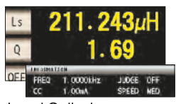
L and Q display screen (1 kHz, 1 mA constant current measurement)
