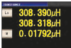
Transformer measurement mode Mutual inductance measurement screen
