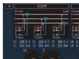
Wiring confirmation function, to avoid wiring mistakes
