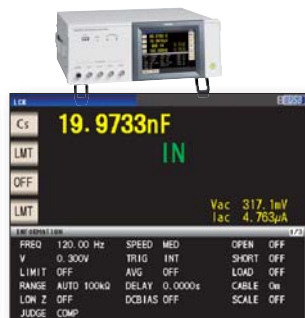
LCR mode Cs display screen (1 kHz measurement)
