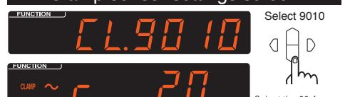
From the menu's clamp sensor selection screen, select the name of the sensor with the cursor key and press the **ENT** key. Then, select the same range as you set for the sensor with the cursor key.
